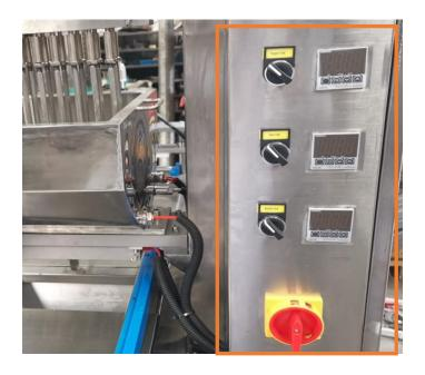
3.4 Depositing is driven by cylinder, control the depositing amount by adjusting the piston travel. (click here to see how to set the depositing amount)
