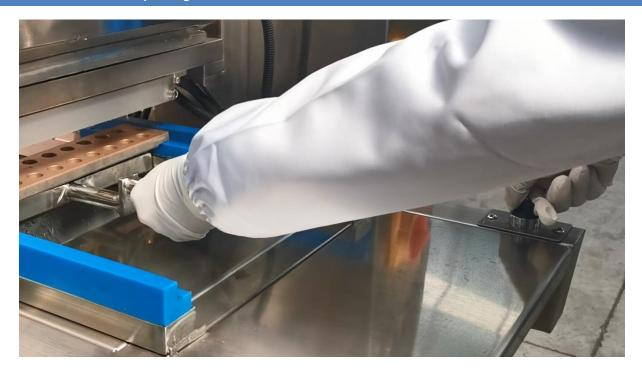
3.8 Take out the mold and put it aside until the gummy solidate. (This normally takes 5-8 minutes). Repeat depositing by using empty molds.
